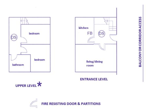
1. All doors separating the entrance hall from rooms at entrance floor level to be fire resisting (minimum 20 minutes) and fitted with self-closer.
