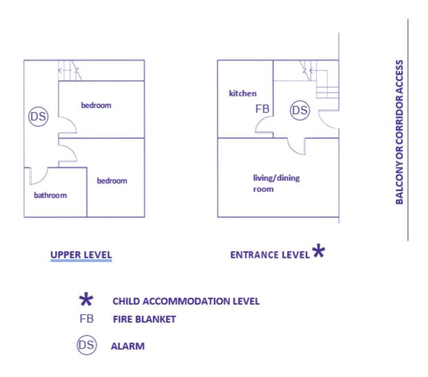
Install mains powered smoke alarms in ground floor entrance hall and upper 1. floor level.
